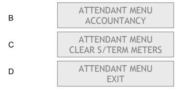
To exit Attendant Menu, use buttons 1 or 2 to move to screen D. Press button 3 to return to normal operation.
